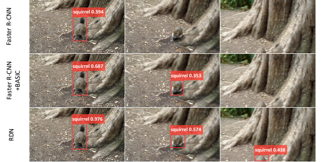
Figure 3. Examples of video object detection results by different ways of relation modeling in our RDN.
